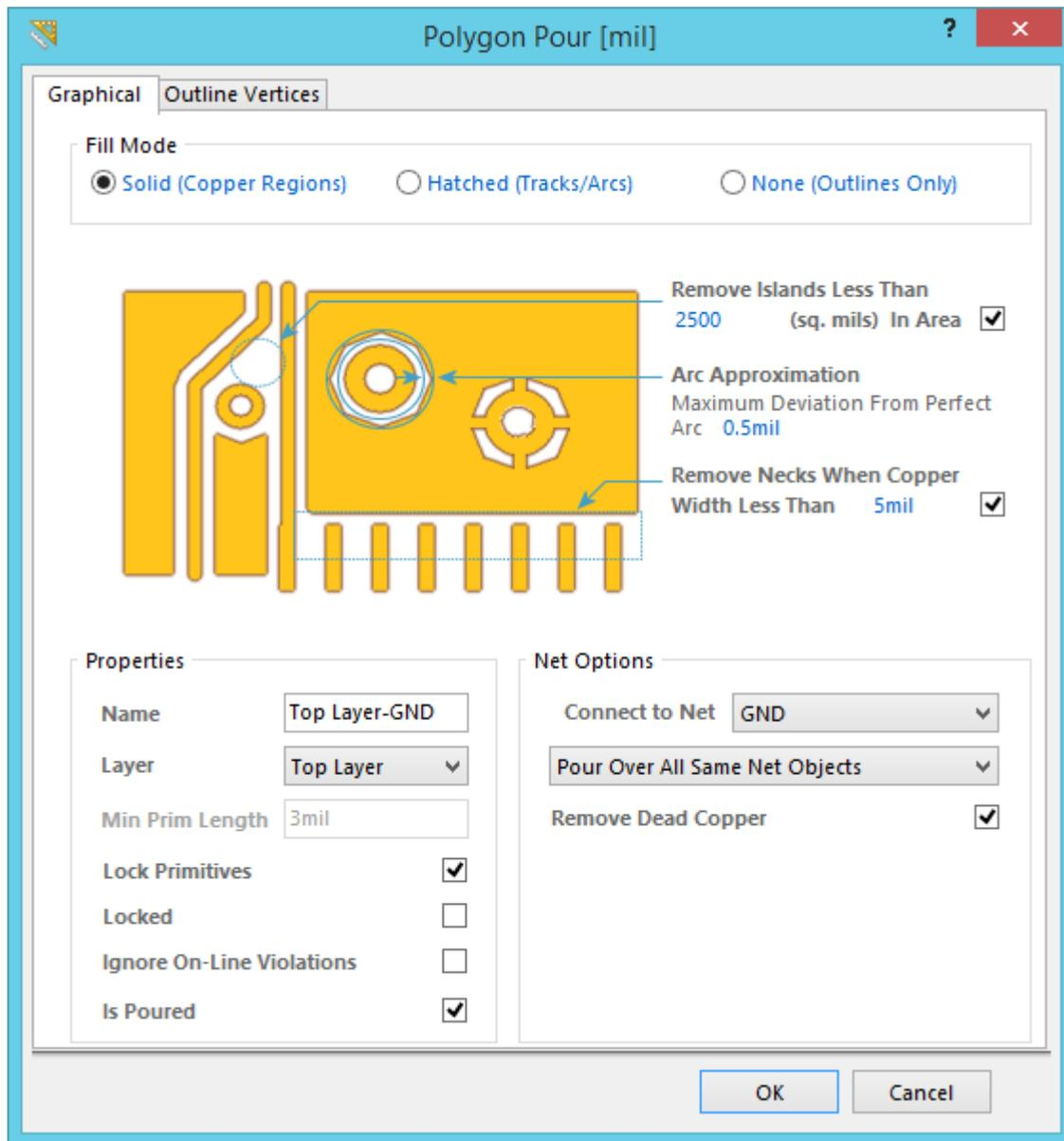
Define the properties of the Polygon before placing it.
