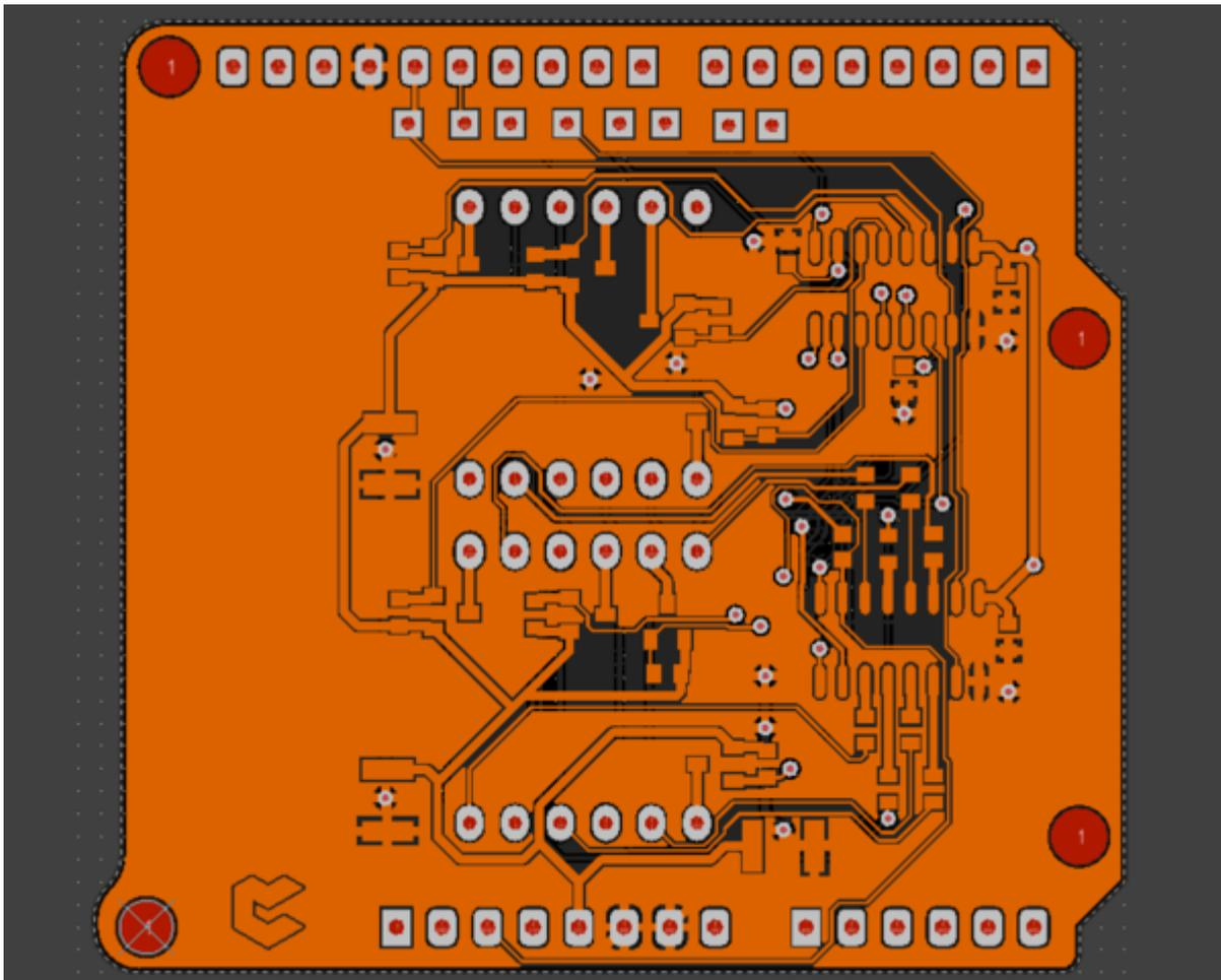
A Polygon Pour being used to create a large GND area on a board.
