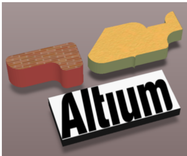
A texture or logo can be added to an extruded 3D Body object.
